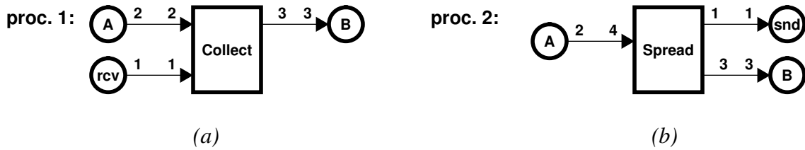
Figure 12. Sub-universes created for processing elements based on the schedule of figure 11. Special blocks, Spread and Collect, are used.
